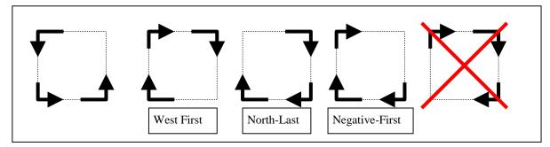
Given the counter-clockwise pattern on the left, we can eliminate three of the four corner turns in the clockwise pattern shown on the right for deadlock-free routing. If we eliminate the remaining corner turn depicted on the far right, it is possible to deadlock in a figure-8. Here, the three right turns are equivalent to the missing North-to-West left turn in the counter-clockwise pattern on the left, completing the cycle.
