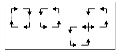
By limiting the possible turns, we can guarantee that a given channel does not have cycles, and is therefore deadlock free. For the 2-D torus, depending on which turns we eliminate, we can create three different deadlock free routing patterns.
