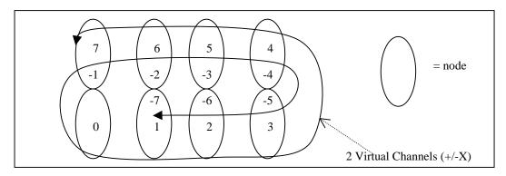
We can jump back and forth between C1 and C2 and still route traffic deadlock-free if C1 is deadlock free across R. This is because we can always make forward progress-- even in the case of blocking on C2 we can then jump to C1 and continue. We are constrained in C1 by a partial ordering on the dimensions and nodes. In the example we used dimension ordering routing which is acyclic and is defined over C1 as:
